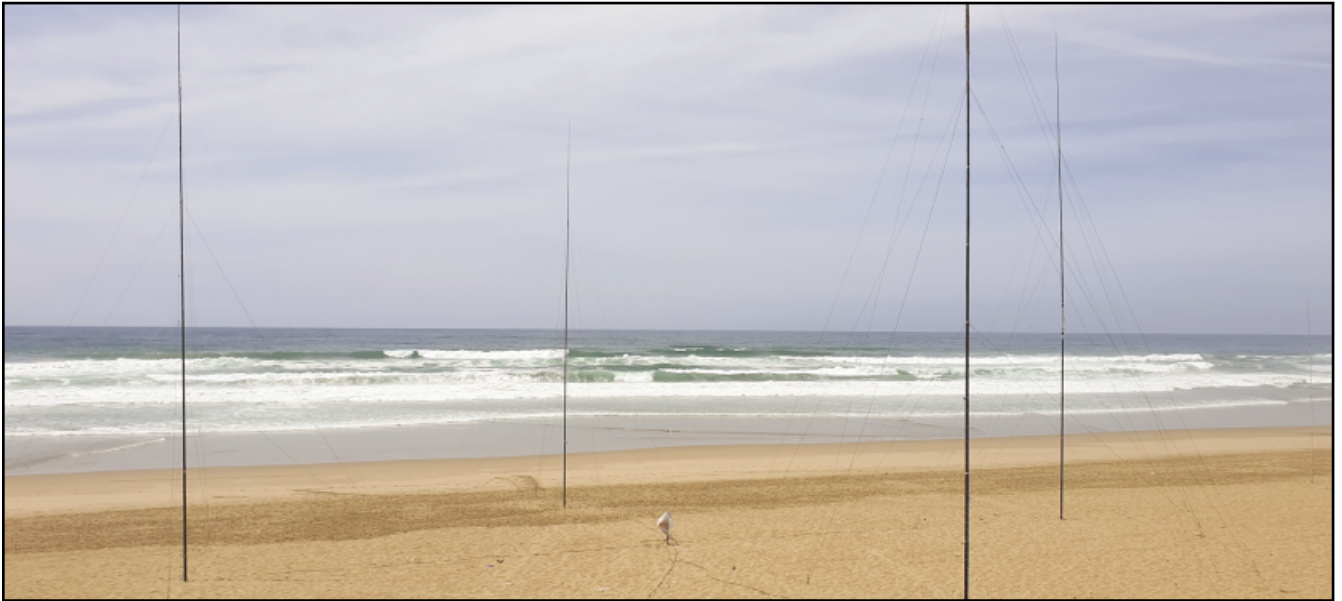
The 80-meter, 4-square antenna at CN2CO is enjoying the Mediterranean beach while Dimitri, RA3CO, is busy operating the contest.
